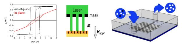
**Left:** Hysteresis loops of a 5  $\mu$ m thick NdFeB film; **centre:** local patterning of a hard magnetic film using the TMP technique; **right**: PDMS  $\mu$ -fluidic device with integrated  $\mu$ -magnets for particle manipulation.
