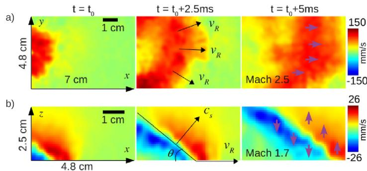
Figure 1: a) observation of a supershear rupture propagating on a homogeneous interface and b) observation of the shock wave radiated by a supershear rupture
