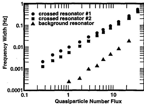
Figure 2: Graph to show comparison of damping on crossed and background resonators.
