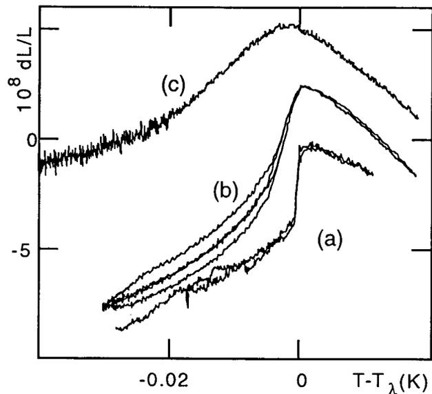
Figure 1 : Length change of three N-aerogels filled with liquid He.  $\rho =$ (a) 0.16, (b) 0.23, (c) 0.36  $\text{g/cm}^3$ . For (b) the raw data is shown before the correction for fountain pressure.
